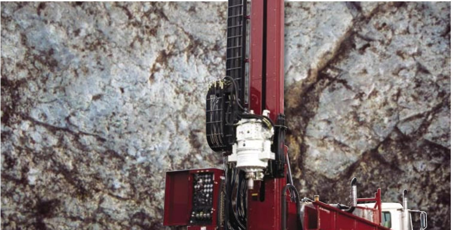
**Sonic** drilling is an innovative new way to drill holes faster and easier than conventional methods. This advanced drilling technology fluidizes and displaces soil particles away from the drill bit and sides of the drill pipe. This allows for clean, rapid penetration rates in a variety of geological formations to depths in excess of 500 feet. Sonic drilling also provides outstanding ability to provide truly representative continuous cores in most geological formations.
